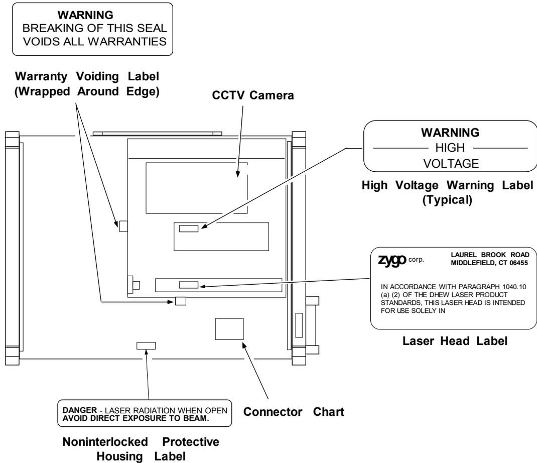
Mark II Mainframe (Top View) with Cover Removed
