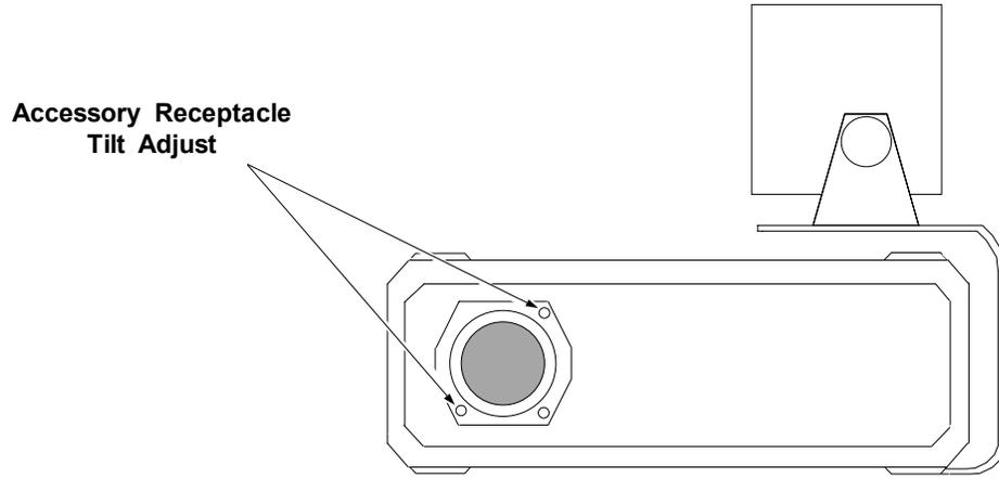
Mainframe Controls - Side View
