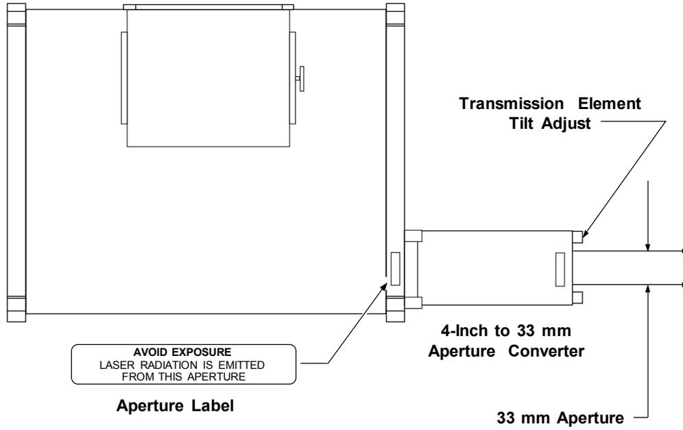
Mark II Mainframe (Top View with Aperture Converter Installed)
